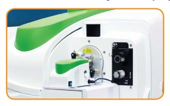
The PC³ is a small, robust Peltier cooled cyclonic spray chamber. The PC³ offers the advantages of low memory effects, constant temperature, fast rinse-out and high sample transport efficiency. The cooled outer walls of the PC³ spray chamber enhance long-term signal stability, reduce polyatomic interferences such as oxides and reduce solvent loading when volatile organic solvents are analyzed.
