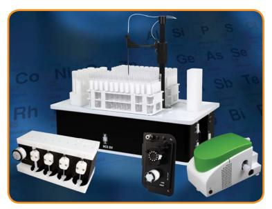
SC-2 DX micro FAST S4 system for organic solvents and low flow applications. The PC<sup>3x</sup> heats the spray chamber to improve sample transport efficiency and sensitivity at low flow rates.
