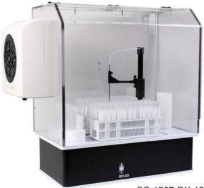
SC-1207-DX-1200 Enclosure with SC-2 DX autosampler
