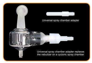
The universal spray chamber adapter is used to connect the hydride gas/liquid separator to any spray chamber.
