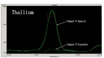
Wavelength scans from a radial ICP-AES of 10ppm solution of As, Pb, Se and Tl introduced with both standard cyclonic spray chamber and the Apex E sample inlet system.
