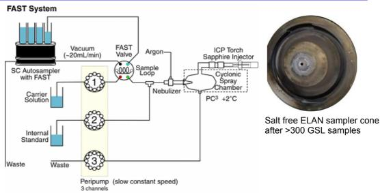
Sample Flow rate: 300µL/min ICP-MS: PE ELAN DRC Internal Standard: Rh. on-line addition Forward Power: 1600W
