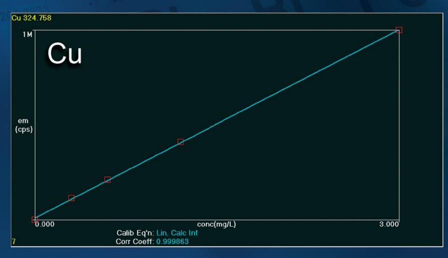
data collected on PerkinElmer Optima 5300 DV
