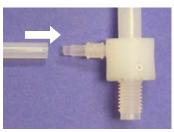
Make sure the gas line is completely on the nebulizer.
